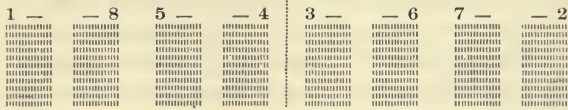
50 Eight pages in quadruplicate, or "four on." Sheet turns on short cross. Produces eight copies.
